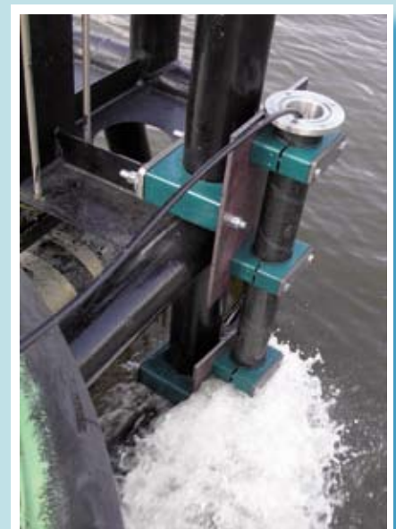
Transducer mounting at typical survey speed
